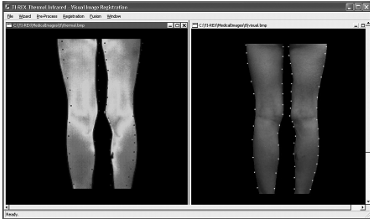
Figure 4. Example of landmark-based registration. Control points have been set for the visual image and copied over to the infrared image.
